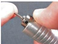
For closing the jaws around a smaller shaft, there's a neat trick. Hold the new bit in the center of the open jaws of the chuck, put your thumb lightly onto the outer toothed collar of the chuck, and gently start up the Foredom. As the chuck turns, it will naturally tighten the jaws around the bur shaft or the drill bit. Then all you have to do is a final tightening with the key.
